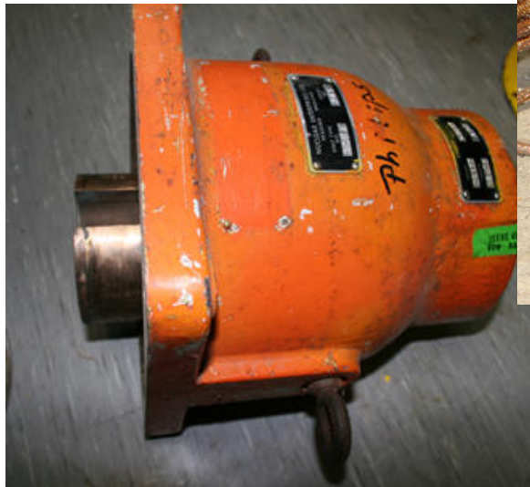
Level indicator (370 MBq Cs-137; 110 MBq Co-60)
