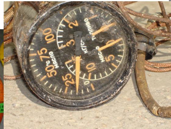
Display device (500 kBq Ra-226; ~ 50 \mu Sv/h at contact)
