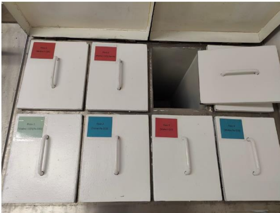
Figure 2: View of the wells where the radioactive waste is placed in along the color-coded tags described in Figure 1, which specify the kind of waste and radioisotope
