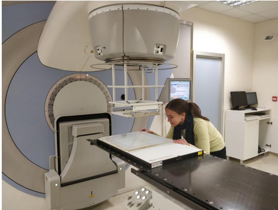
Figure 2. Demonstration of quality control of a radiotherapy linac during hospital placements
