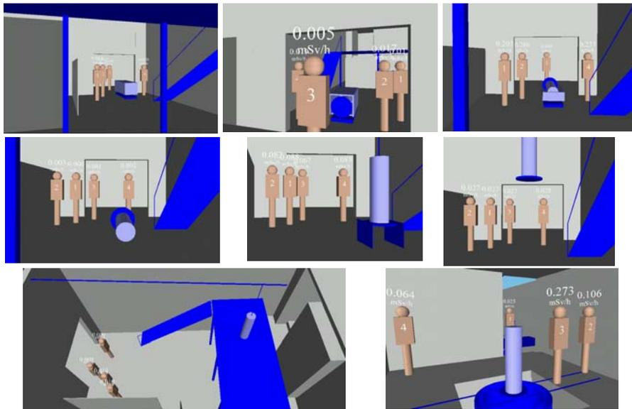
Fig. 1. Simulation of the spent fuel loading operation using VISIPLAN 3D ALARA planning tool.
