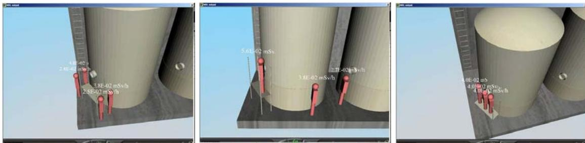
Fig. 2. Simulation of the cleaning of the high level waste tanks at BR3 (from left to right the placement of the scaffolding, the placement of the high pressure cleaner and the cleaning operation with a gradually reducing source strength).
