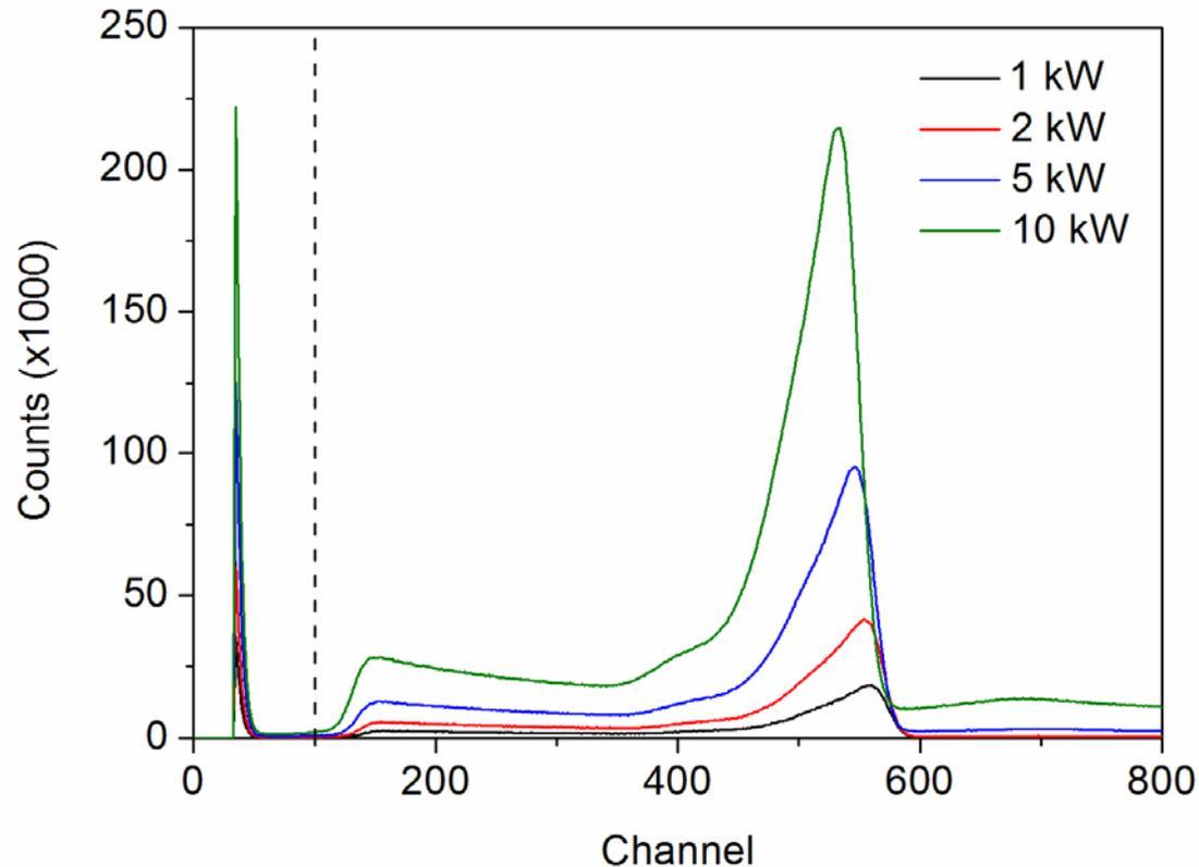
Signals due to gammas and neutrons have different amplitudes.
