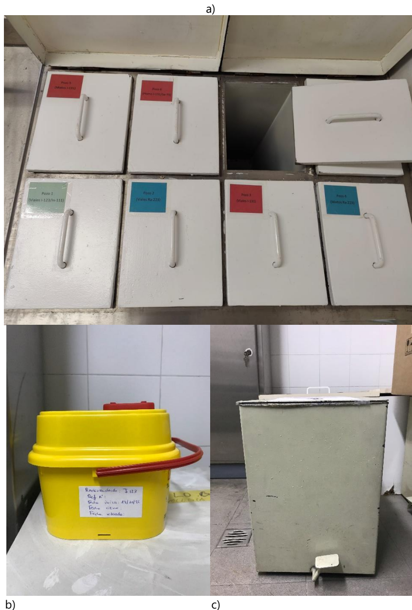
Figure 3: Pictures of the different places for storing radioactive waste. a) Wells (vials and mixed waste); b) Yellow box (syringes); c) Shielded bin (mixed waste).
